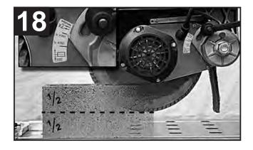
By means of the cutting square, arrange the piece to be cut on the working table at the desired measurement. - Start the machine and carry out the first cut (see picture 19).
